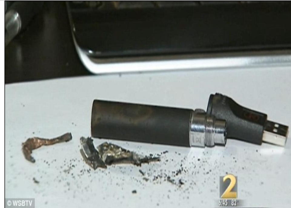
Scorched: The Chinese-made eHit electronic cigarette was charging in a computer USB port when it exploded
